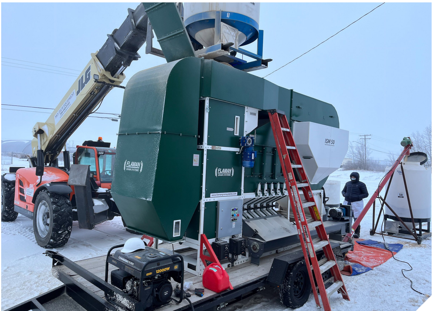
Air fractionation machines like the one shown here use air flow to separate lighter, DON-infected barley from healthy kernels.
