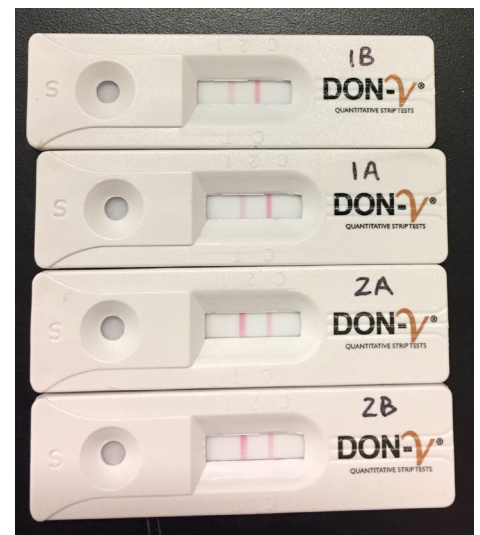
At the Canadian Feed Research Centre at the University of Saskatchewan (top), new and improved animal feeds are researched, developed and commercialized. (Right) Strip tests can measure total DON in grain at levels as low as 0.20 ppm.
